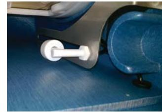
Take out the rubber plug from the housing and pull out the level switch connector. Push the connector through the rubber plug so it is free.
