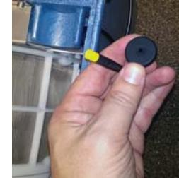
Remove the level switch from the drum chamber by taking the nut and connector through the mounting bracket.
