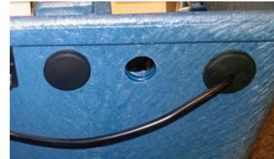
Push the connector through the mounting bracket in the inlet chamber. Please keep in mind that the level switch must be rotated 180 degrees in regards to the gravity position! Then put the nut over the connector and screw it on the level switch.
