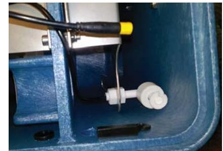
Push the connector through the opening and push it through the rubber plug. The small hole of the plug can be widened with a sharp knife to make this a little easier. Put the plug in the middle opening.
