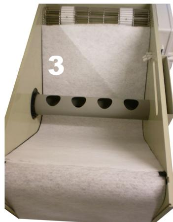
Put the 2 separate lengths of roll in the filter (3). (Not under the rubber guidance strips).
