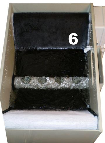
The level switches will activate the conveyer belt motor and the fleece will now be transported automatically (6).
