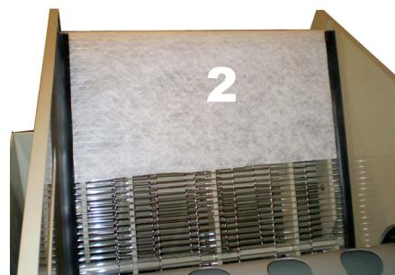
Feed the fleece membrane from the roll for about 30 cms under the guidance strips (2).
