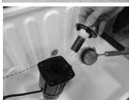
Remove rotor from pump house and clean with water and brush
